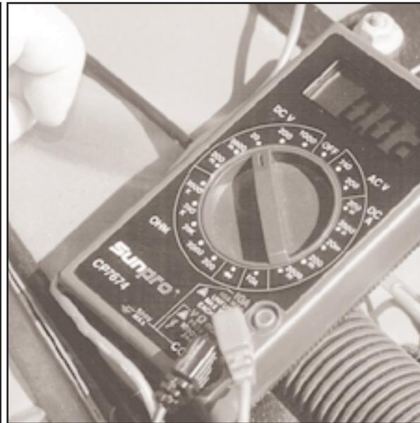
After turning your digital volt-ohm meter to DC volts, touch the negative connection to the battery (left). Next, dip the positive lead into the coolant at the filler neck (center). Be sure not to touch the sides or bottom of the radiator with the lead. Finally, look at your reading (right). Anything over .10 volts is cause for concern.
