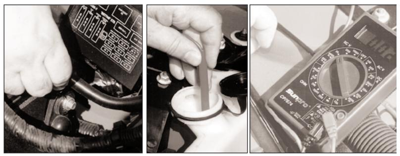
After turning your digital volt-ohm meter to DC volts, touch the negative connection to the battery (left). Next, dip the positive lead into the coolant at the filler neck (center). Be sure not to touch the sides or bottom of the radiator with the lead. Finally, look at your reading (right). Anything over .10 volts is cause for concern.
