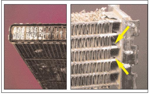
Stray current inside the cooling system can cause excessive corrosion of metal components (left) as well as an electrochemical reaction that will produce voids in radiator tubes. Photos courtesy of Modine Manufacturing.
